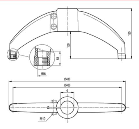
$\begin{array}{ll} \text{d (inch)} &= 2 \text{ Gas} \\ \text{d mm} &= 60.3 \\ \text{Weight (g)} = 650 \end{array}$
